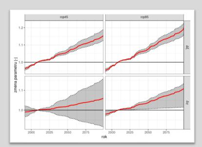
Change of GEV model parameters for hourly precipitation extremes. The gray area shows the range between 25% and 75% quantile, the red line the average.
